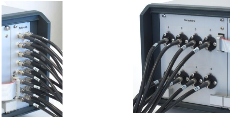
Figure 3: Fiber optic connections on the source coupler unit (left) and detector unit (right).
