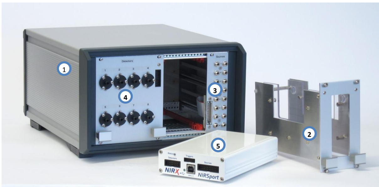
Figure 1: NIRSport APD/LED coupler module and main components: (1) Main frame; (2) NIRSport cradle; (3) illumination unit; (4) detection unit; (5) NIRSport.
